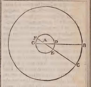
In the Diagram set down before, if we suppose F, to be the place of the power, and C of the weight, the point A, being the fulciment or center, then in the same space of time, vvherein the power does move from F, to G, the weight will passe from C, to B. These distances having the same disproportion unto one another, as there is betwixt AF, and AC, which is supposed to be quadruple. So that in this example, the weight vvill move four
